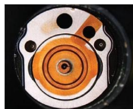
At Start: Deposits in Injectors
